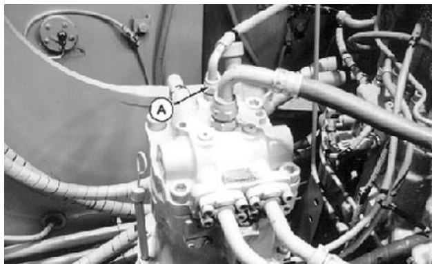
A—Swing Motor-to-Hydraulic Oil Tank Drain Line
