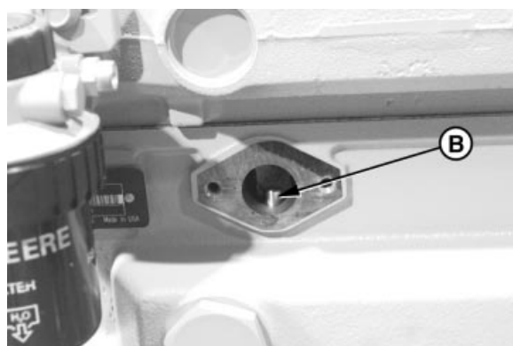
B—Pump Actuator Pin C—Magnetic Follower Holder Kit
