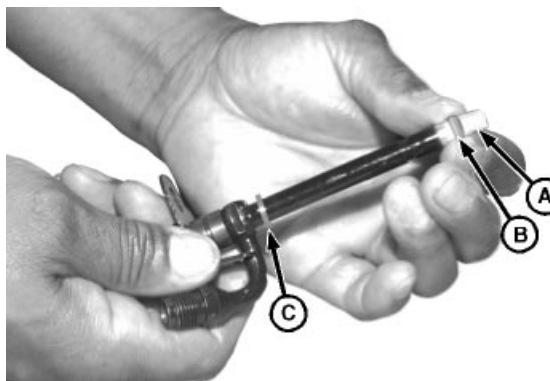
A—Pilot Tool B—Carbon Stop Seal C—Seal Washer
