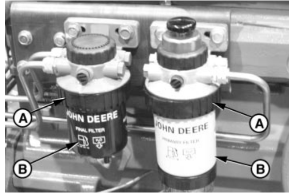
A—Retaining Ring B—Filter Element
