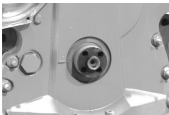
A—JDG954-2 Adapter B—JDG954-1 Installer C—Oil Seal
