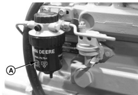
A—Final Fuel Filter B—Primary Fuel Filter/Water Separator
