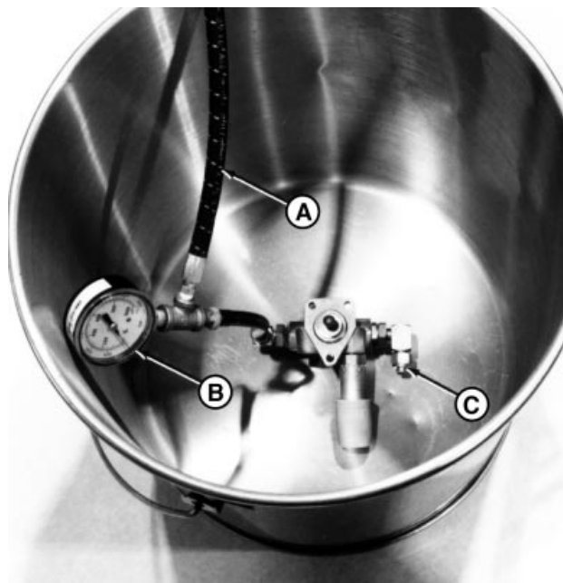
A—Air Line B—Pressure Gauge C—Outlet Fitting
