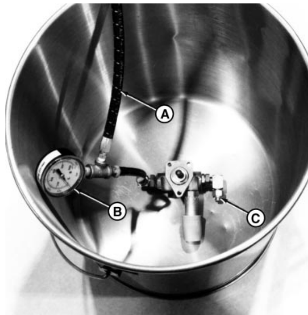
A—Air Line B—Pressure Gauge C—Outlet Fitting
