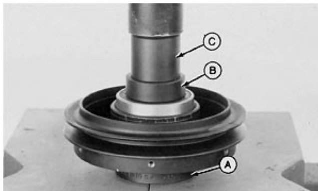
A—Bearing Support B—Bearing Adapter C—Pulley Adapter
