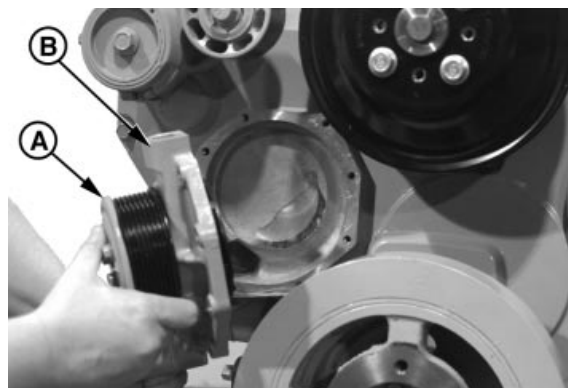
A—Pulley B—Water Pump
